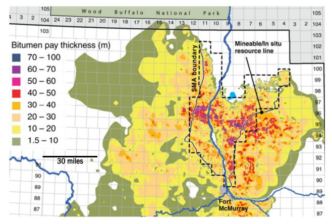
**Figure 83. Distribution of bitumen pay thickness in the Wabiskaw-McMurray Deposit.**<sup>174</sup> Bitumen pay thickness is a proxy for resource quality. The cutoff line separating surface mineable deposits (SMA) and in situ deposits is indicated. As can be seen, the thickest pay is located in the surface mineable area and is relatively localized.
