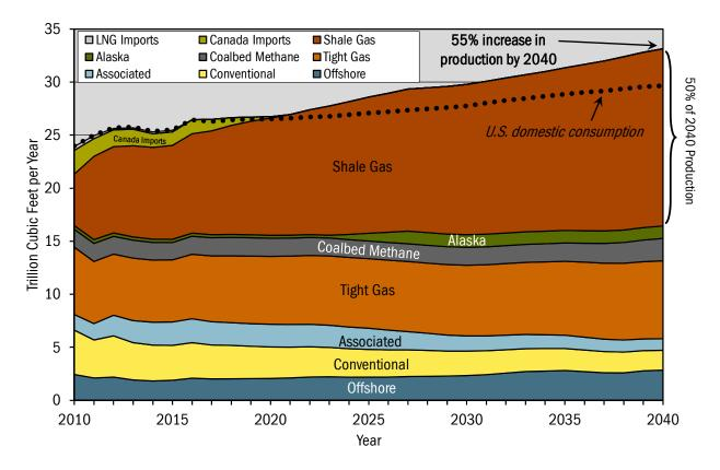
**Figure 32. U.S. natural gas supply by source, 2010-2040 (EIA Reference Case, 2013).**<sup>60</sup> Shale gas accounts for 50 percent of production in 2040.
