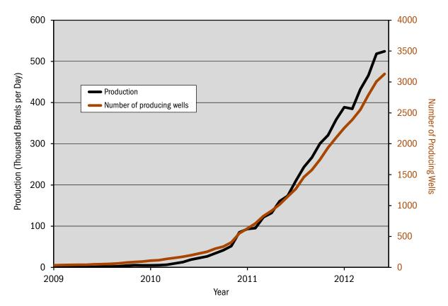
Figure 71. Petroleum liquids production and number of producing wells for the Eagle Ford shale play, 2009 through June 2012.<sup>148</sup>
